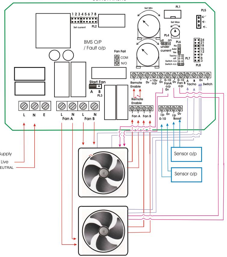
This connection shows a DC fan connected up with a zero to ten control input along with an enable.
